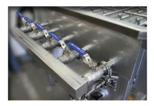
Individual valve zone control for washing at less than full capacity.
